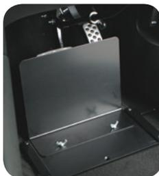
The hinged accelerator pedal and pedal guard are not suitable for all vehicles. **To check compatibility call our support team on 0161 430 2151**
